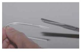
You should be left with a tapered end to the tubing.
