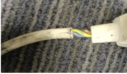
Exposed Inner Cores, the outer sheath is not held by the cord grip
