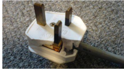
Cracked plug with exposed live terminal
