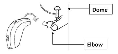
Please note the image shown is for a right hearing aid. For the left hearing aid, the dome would be facing down when the elbow has been turned at 90 degrees anti-clockwise.
